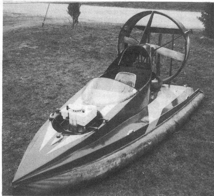
UH-15P with thrust duct
